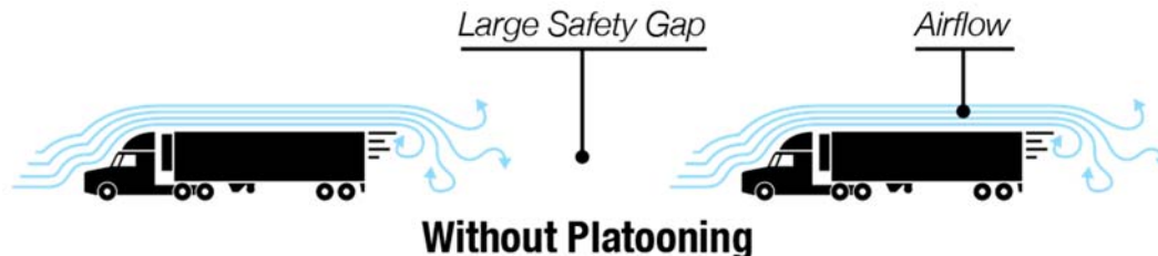
Figure 3.2 Explanation of Truck Platooning Efficiency Benefits
